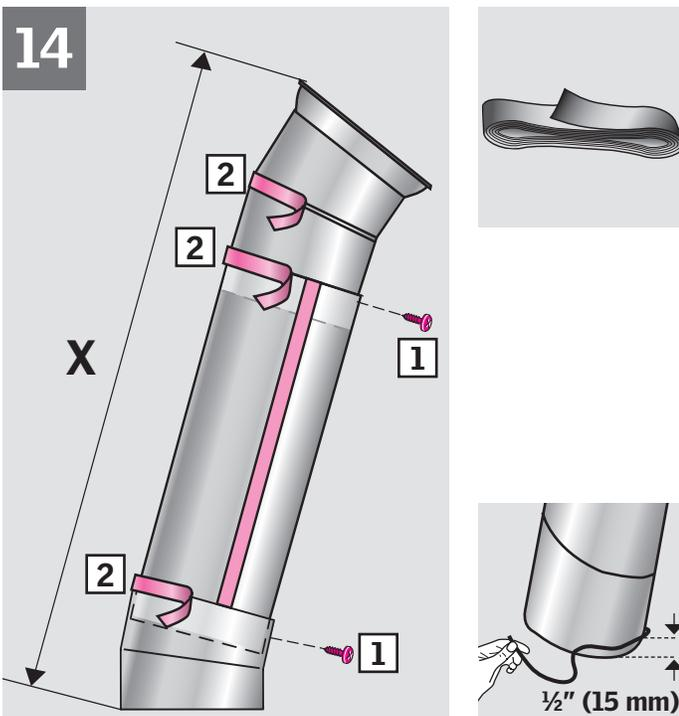
**English:** Connect the straight tunnel sections with elbow(s), fitting the straight tunnel section to go on the outside of the upper elbow and inside the lower elbow.
