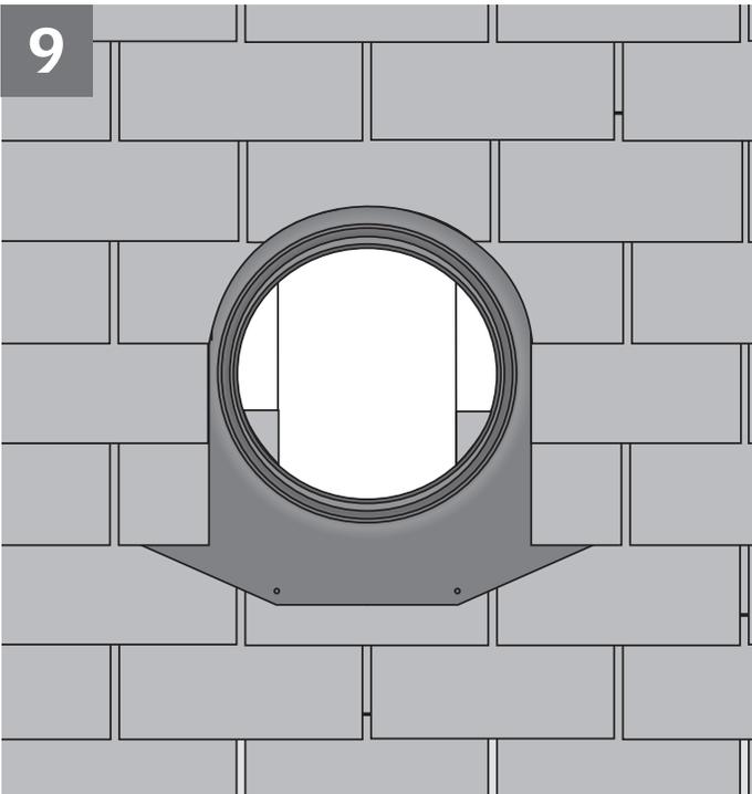
**English:** Reinstall roofing material over the flange. Leave a  $\frac{5}{8}$ " (15 mm) channel for water to run off. Optional ZTA turret extensions available where domes need to be elevated by 6  $\frac{1}{2}$ " (165 mm), or 9" (230 mm).
