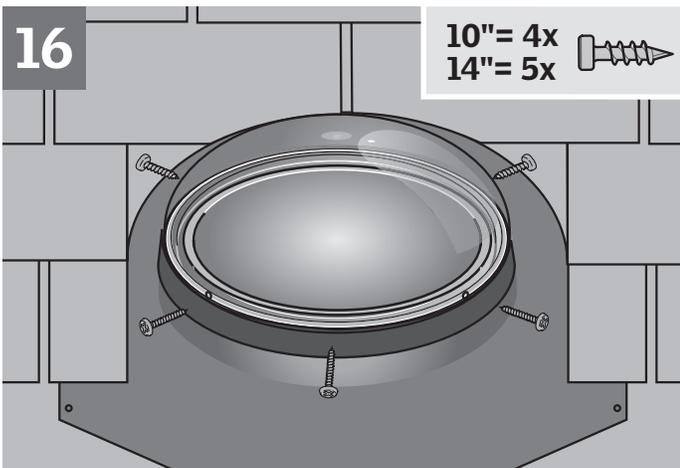
**English:** Align holes and install and secure the dome with the ¾" (19 mm) screws provided.
