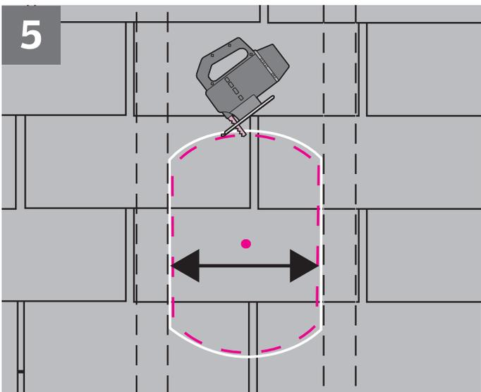
**English:** Mark the sides of the rough opening and cut rough opening. **CAUTION:** Be careful not to damage any framing members.
