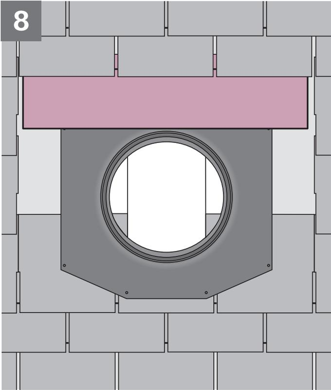
**English:** Overlap the top of the flange with underlayment to allow for proper drainage.
