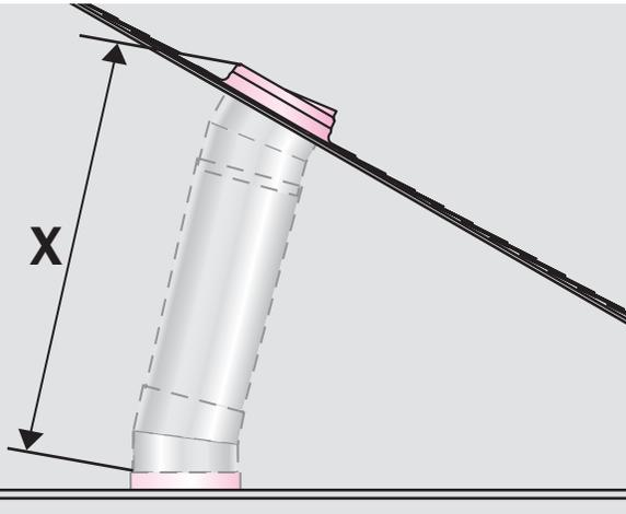
**English:** Determine the overall length of the straight tunnel section. Include minimum 3" (80 mm) to overlap the elbows and minimum 1½" (40 mm) for each additional straight tunnel section.
