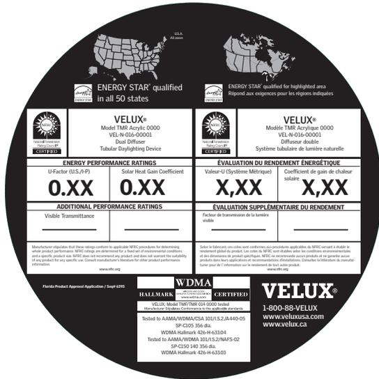
**English: If seeking building code approval,** attach the **NFRC** label (provided at product) to the visible area of the ceiling ring and diffuser. The NFRC label must be visible from the interior room during the inspection process.
