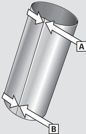
**English:** Remove protective film and assemble the straight tunnel sections to go outside the upper sections and inside lower sections. At upper end of tunnel sections, align the notches to create a wide tunnel opening **A** and at bottom of tunnel sections, align the notches to create a narrow tunnel opening **B**.
