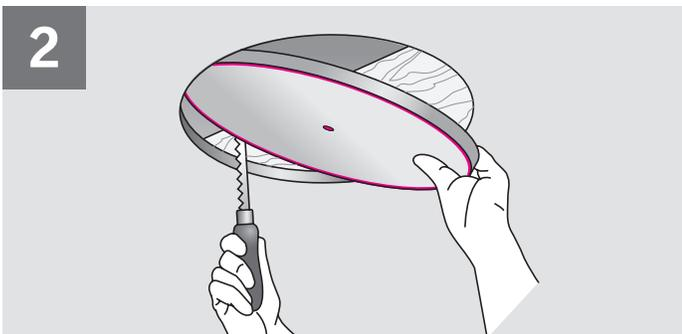
**English:** From inside, locate the nail indicating the center of the SunTunnel in the ceiling and mark circle and cut hole in the ceiling as shown.
