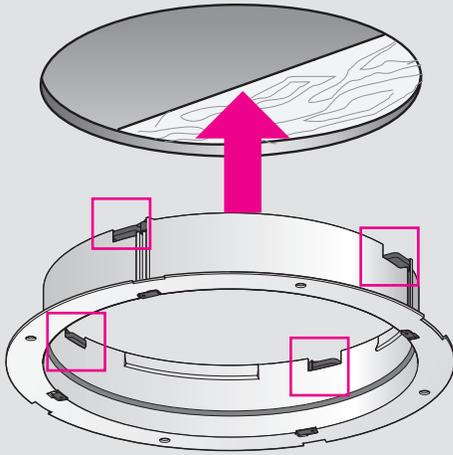
**English:** Rotate the plastic "plates" into hidden position and insert and secure the ceiling ring, insuring a tight joint between the ceiling ring and the ceiling.
