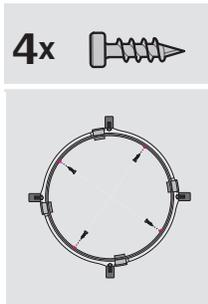
**English:** Secure tunnel assembly to ceiling ring with four of the  $\frac{3}{8}$ " (10mm) screws provided.
