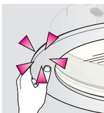
**English:** Install the trim ring by centering under the ceiling ring and snapping the four to six tabs into position. Or the tabs can also be aligned with the notches and then rotated to secure.
