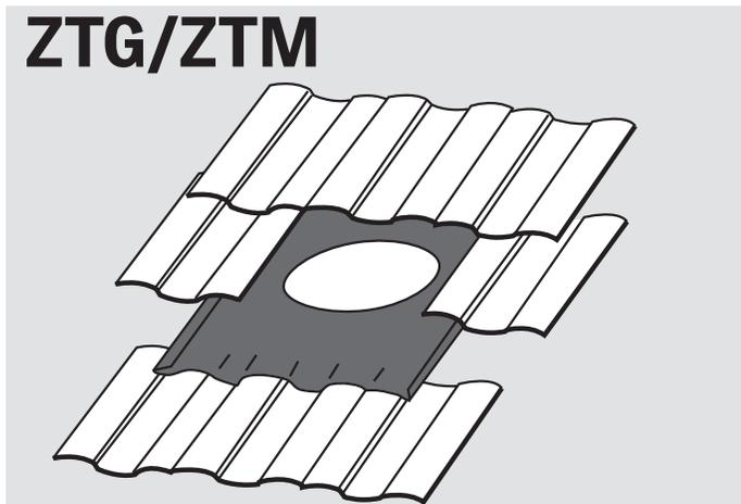
**English:** Sun Tunnel tile roofing - Refer to type ZTG/ZTM tile kits for installation in tile roofing.
