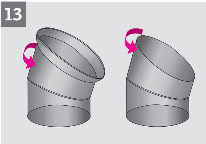
**English:** Adjust angle of both elbows. Elbow can be damaged if excess force is applied.
