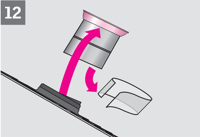
**English:** Install the pivot ring on the upper elbow and remove the protective film.
