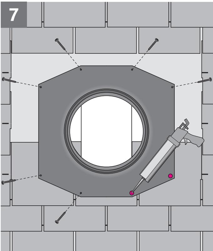
**English:** Center the flashing over the rough opening and secure the flange with the provided 1 ½" (40 mm) screws in all the pre-punched holes along the edges. Seal all exposed fasteners.
